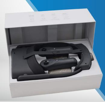
The VF2000 NEO is a first-of-its-kind, portable tool, able to perform the comprehensive visual field analysis of the VF2000, like the 10-2, 24-2, 30-2, Estermann test (and more), five core vision tests, and has the added ability of **Active Eye Tracking:**
